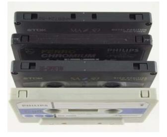
**Type IV:** tapes referred to as "metal", it can be identified by the wider write protect tab hole and extra holes in the center of the tape.
