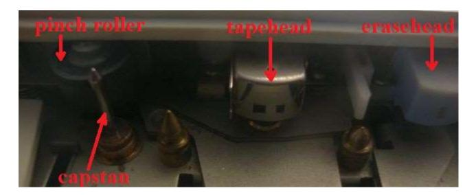
So in other words... always make sure that your datasette (or other kind of tape recorder) is in perfect working condition. A backup or restored tape is only as good as the recorder is was made on. If you use a crappy recorder, you'd get crappy recordings!
