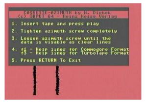
speed loader, in fact the actual data on the tape doesn't really matter, as long as it is there long enough for you to calibrate the tapeheads. If the tape is too short, you'll be constantly rewinding the tape, which could be a bit unpractical.
